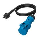
3-core rubber sheathed cable 1.5 m long with CEE connector 16A, 3p, 230V and plug SCHUKO® 16A, 230V
