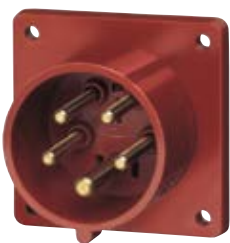
Panel mounted phase inverter inlet flange 75 x 75 mm, fixing distance 60 x 60 mm, a retaining nose to hold the hinged lid of the connector must be provided by the customer in order to ensure satisfactory locking
